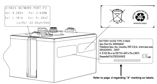
Figure 2-10 2196EX battery module and labeling
